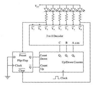
Assuming that the initial value of counter output (Q<sub>2</sub> Q<sub>1</sub> Q<sub>0</sub>) as zero, the counter outputs in decimal for 12 clock cycles are
