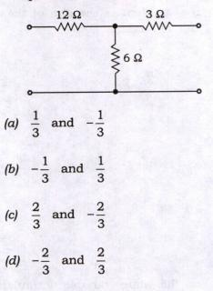
**53.** What are the open-circuit transfer admittance and the negative shortcircuit current ratio respectively for the two-port network shown in the figure?
