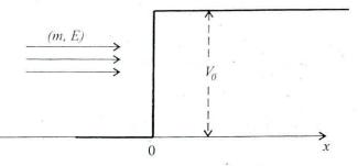
A beam of particles of mass *m* and energy *E* is incident on a step potential of height  $V_0$  from the left as shown in the figure. Discuss the behaviour of the particle for (i)  $E < V_0$  and (ii)  $E > V_0$ . Obtain expressions for the reflection and the transmission coefficients and sketch them as a function of the incident energy of the particle.
